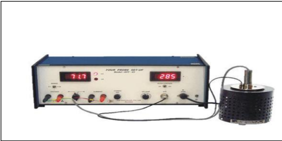
Fig. Energy band gap by four probe method with pc interface .
